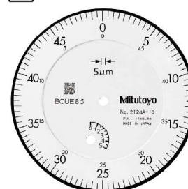
Graduation: 0.005 mm, Measuring range: 5 mm
